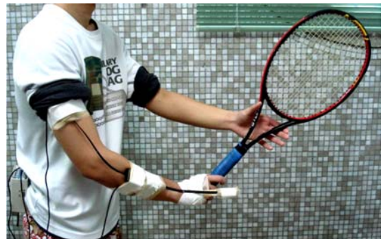
Figure 1: Posture measured by joint angle sensor.
